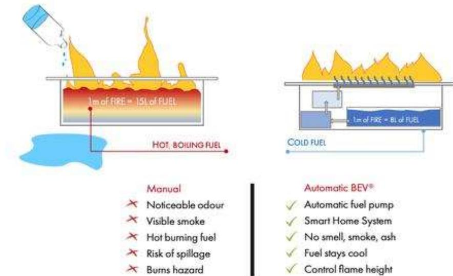
Automatic BEV® technology guarantees complete separation of the fuel tank and fire. This, coupled with multiple sensors, meets even the most robust safety requirements.
